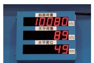
A display allows workers to check the system status during testing.
