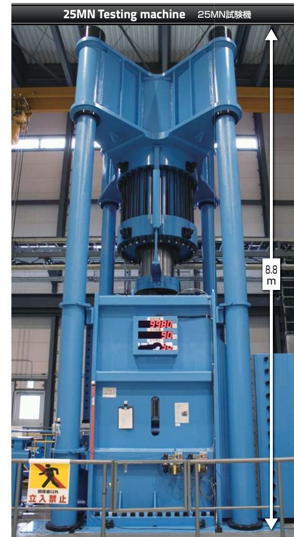
PILLAR has installed a biaxial tester (reciprocating sliding tester) capable of accommodating compression force loads of 25 MN (2,500 t), making it one of the industry's leading seismic isolation testers. The system is utilized primarily in testing to evaluate the performance of seismic isolation bearings used in seismically isolated buildings.
